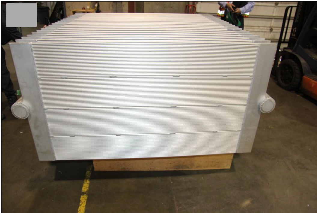
Figure 2 Side plates showing no evidence of deformation.
