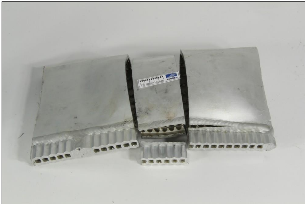
Figure 10 Bulged plate cut to reveal internal construction.
