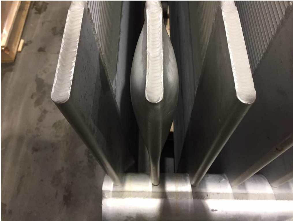
Photo 1: Heat exchanger plate showing bulge deformation on both sides of the plate.
