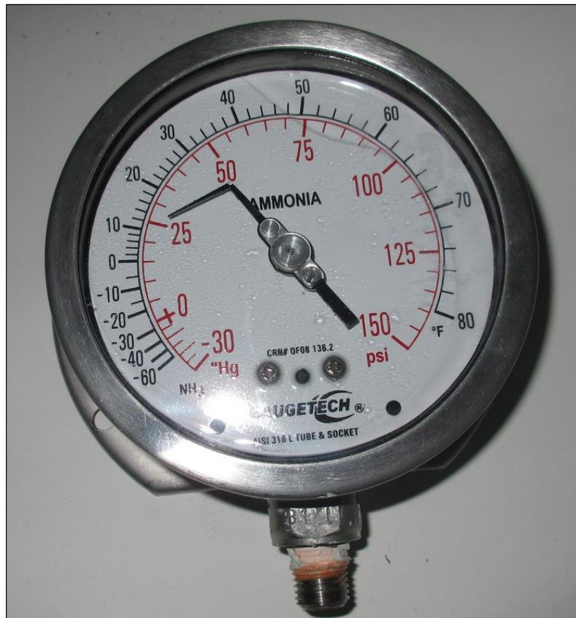
Figure 18 Overall view of damaged pressure gauge attached to cold trap.
