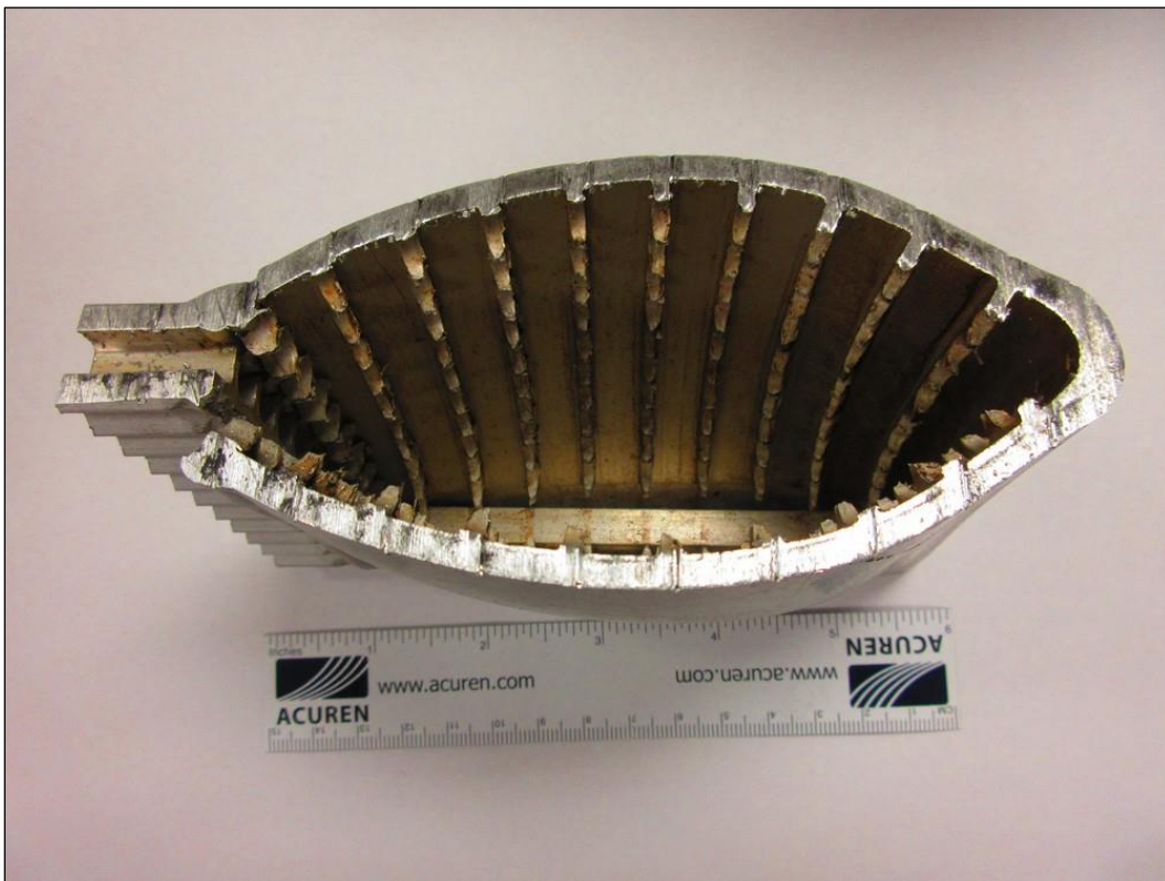
Figure 11 Bulged plate integral surface. The legs between each hole have fractured.
