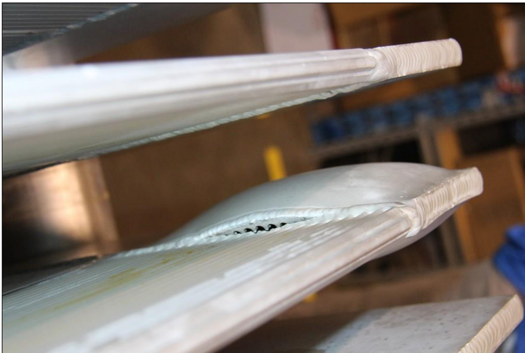
Figure 4 Weld tearing at bottom of bulge. Identical tearing was found on both sides of bulge (see Figure 5).
