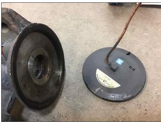
Photo # 2: Approximately 3 inch diameter diaphragm (7.2 sq. in.) with 1/8 inch I.D. copper line attached.
